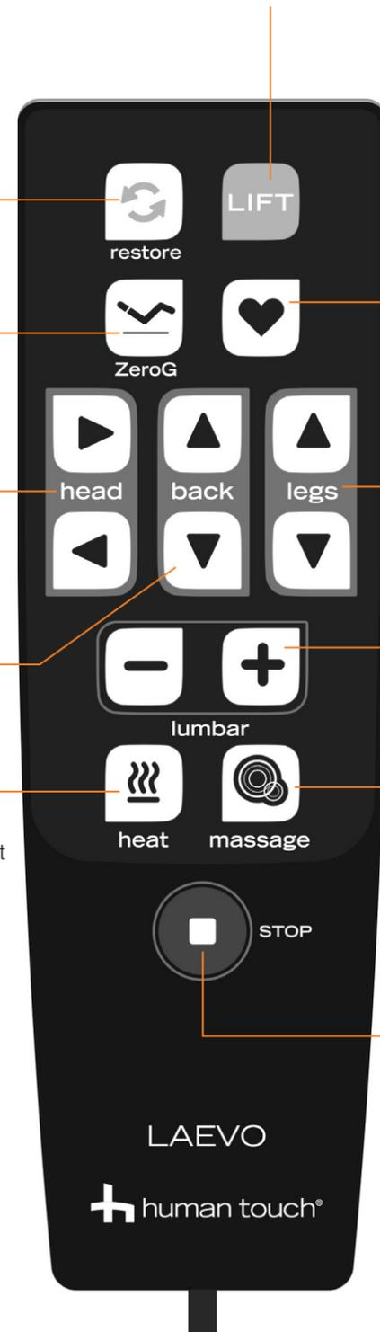
**MEMORY:** To save the chair's current backrest and legrest position for easy recall, press and hold the **MEMORY** button until it flashes blue. Press the **MEMORY** button to recall the saved position.
