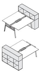
**Bigger Depot** has the ability to turn the top section around so it faces the table top when placed against the end of the Bivi table.
