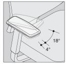
Arms pivot 18° inward and 4° outward on models with adjustable pivot arms. Grasp arm and push front to left or right
