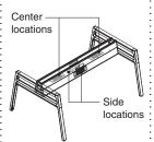
If both locations in the center and both locations in the side of the trough are used for power, there is a total of four power strips available in one trough. A package of four (TS2PS4PK), ordered separately, would allow a total of 16 plugs.
