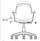
Seat height adjusts pneumatically. To lower, pull lever up while seated. To raise, pull lever up and keep your weight off the chair. Range of adjustability is 51/4" from 16"H to 213/16"H, a 33/4" range (171/8"H to 203/4"H) is available on chairs with a worksurface. Stools are standard with an 81/2" range of adjustability (231/16"H to 313/8"H). A 71/2" range of adjustability (181/2"H to 267/16"H) is available as an option.
