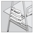
Board Racks can be attached at the bottom location of Tall Arch or a Short Arch.
