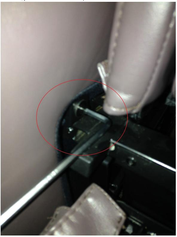
The first thing you should do when removing the panel is to walk beside it and slowly pull it upwards. You will start to see enough room to place your hand inside. Use one hand to totally disconnect the air hose and another hand to hold the panel. Once removing, you can set it off to the side.
