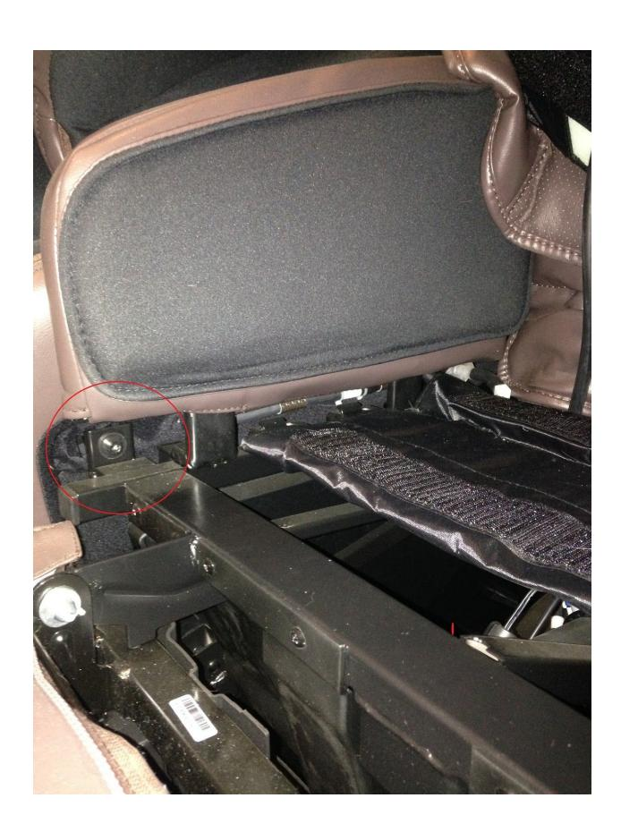
Now start removing the bolt with your Allen Head. This should only take a few minutes. Once it is removed, you will be able to remove the panel.
