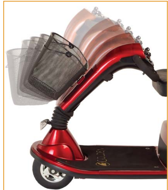
Patented infinite adjustable tiller
